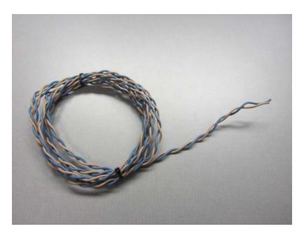
We also terminate both ends of the twisted pair wire by using 120  $\Omega$  terminating resistors at each end to reduce reflection.
