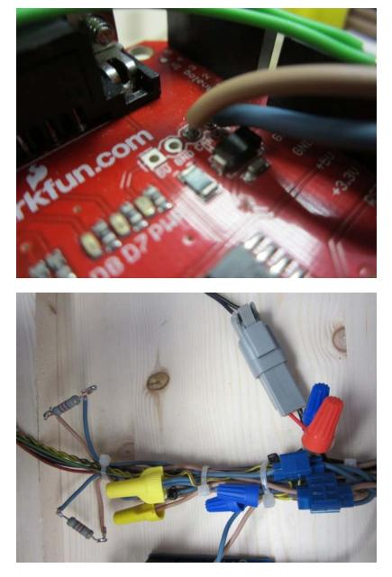
The Arduino will be powered from the same 12V DC power source that powers the instrument cluster. The Arduino Uno features a built in voltage regulator at the power port. Considering the safety benefit of the voltage regulator, applying 12V of power to the Arduino was not an issue as the Arduino Uno specifications explicitly state that the microcontroller can handle a recommended 7 - 12 volts.
