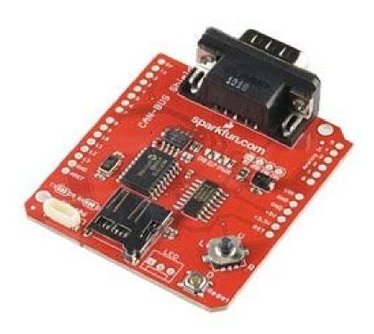
To interface the CAN shield with the data bus, we splice the 18 gauge twisted pair wire from the CAN bus and solder CAN-H and CAN-L wires coming into the pins on the CAN shield.
